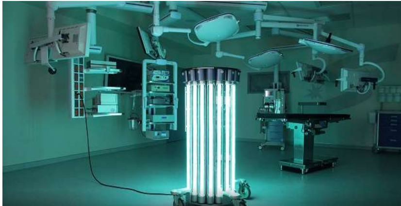
The robots use ultraviolet-C light to deactivate viral cells in the air and on surfaces. They were originally designed to be used primarily in hospitals. (Submitted Photo)
